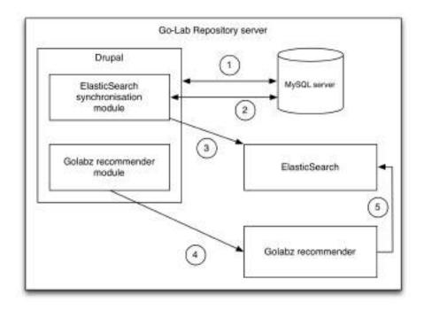
Figure 18. Architecture of the Go-Labz recommender system.
