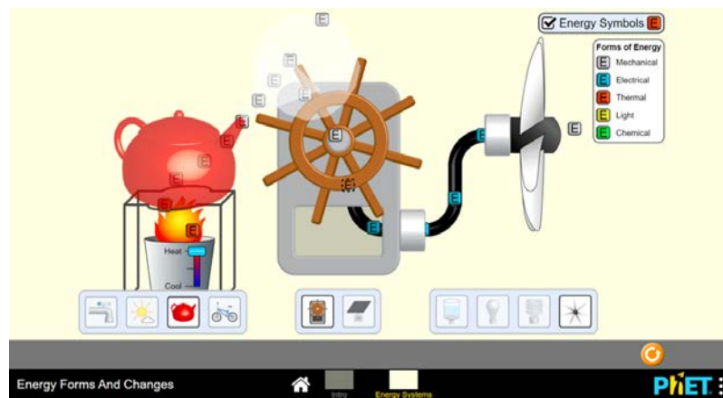
Figure 8. A screenshot of the Energy Forms And Changes lab in which thermal energy (heat under the teapot) is transformed into mechanical energy (rotating fan).
